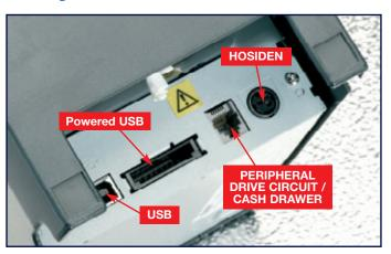
The printer is supplied with two port covers for use depending on configuration chosen.
