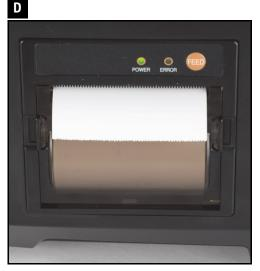
6. To feed more paper, press the **FEED** key on the printer. The specification for the paper is:
