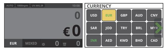
If more currencies are installed than can be shown on one screen, a green arrow is displayed at the right; touch the arrow to scroll to the remaining currencies.
