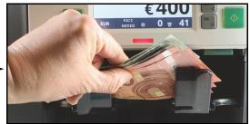
Remove notes from the stacker and reject pockets Feed rejected notes again, if required, to separate notes rejected for different reasons.
