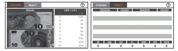
To move between the stacker and reject pockets, touch the **Stacker** and **Reject** tabs. For instructions on viewing detailed **Totals**, see page 45.
