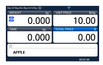
② Place an item on the platter and press the V1 key. This transaction is save to memory.
