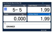
⑤ Press the PRINT key. Markdown(STRIKE THROUGH) is printed on label as figure.
