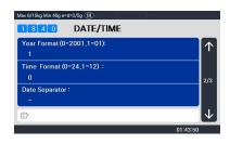
3. Set separators for "TIME", using ASCII code table on page
