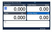
**Note:** - If you set "Label Prt. w.o Rewind (X Key)" to "Y" in menu 1872 of program mode, the scale does not check peel-off, so you have to press FEED key after printing is done. (See chapter 2.14.21)
