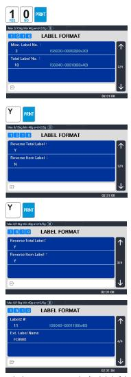
If you do not wish to use the label #2, simply input '0'. It operates in the same manner as the Aux.Label of the PLU input items. If the Aux.Label No. of PLU has already been registered, print with the corresponding label number, and if not, output the inputted Label #2
