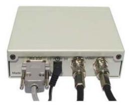
Serial Power Video Video Output Input Input Figure 3: VSI-Pro Cable Connections
