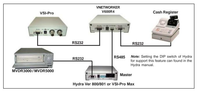
Figure 147: Connection Diagram of VSI-Pro RS-485 Network with MVDR3000/5000
