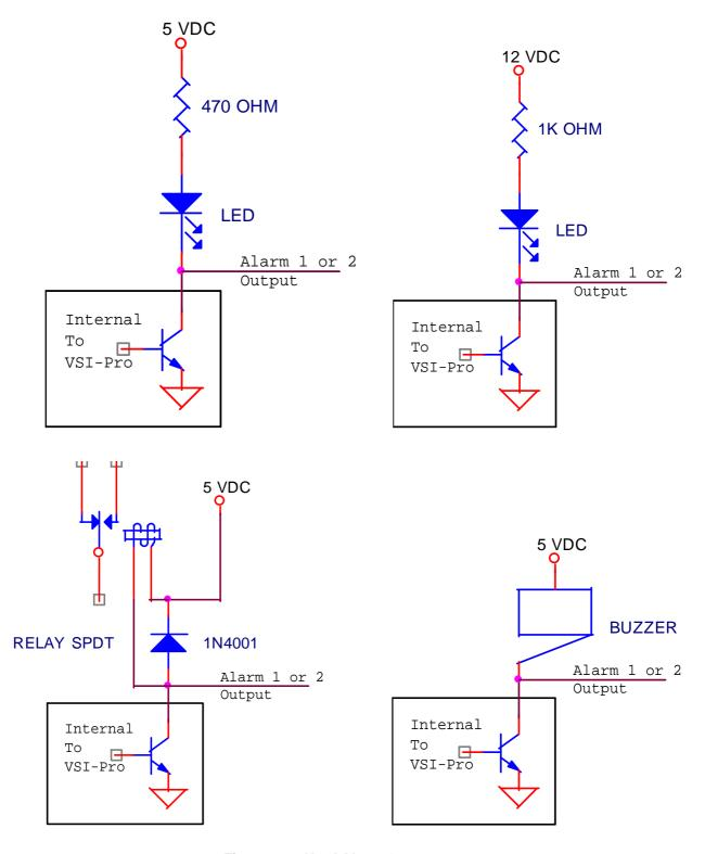
Figure 142: Hard Alarm Output
