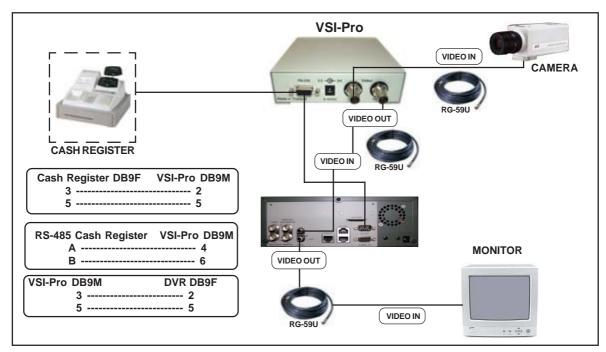
Figure 150: Connection Diagram of VSI-Pro and Cash Register with MVDR3000/5000
