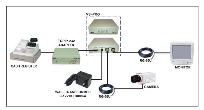
Figure 140: VSI-Pro Connections with TCPIP 232 Adapter
