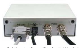
Serial Input Power Video Input Video Output Figure 133: VSIB Connection Cables
