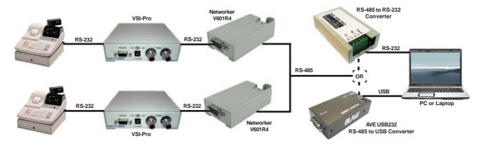
"n" means up to 64 Cash Registers / VSI-Pros / RS-485 Networkers can be connected on one RS-485 Network
