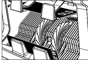
Counting the value and quantity of banknotes sorted per denomination version (divide old and new versions). Banknotes with a different denomination version than the first counted banknote are transported to the reject pocket.
