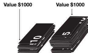
Manually set a desired value. The machine counts banknotes until the desired value is reached. Banknotes not useful in reaching the desired value will be transported to the reject pocket.
